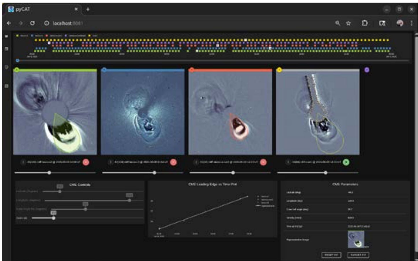
PyCAT user interface, showing multi-perspective coronagraph images from four spacecraft instruments and interactive sliders for fitting these observations to a 3D CME Cone model.
