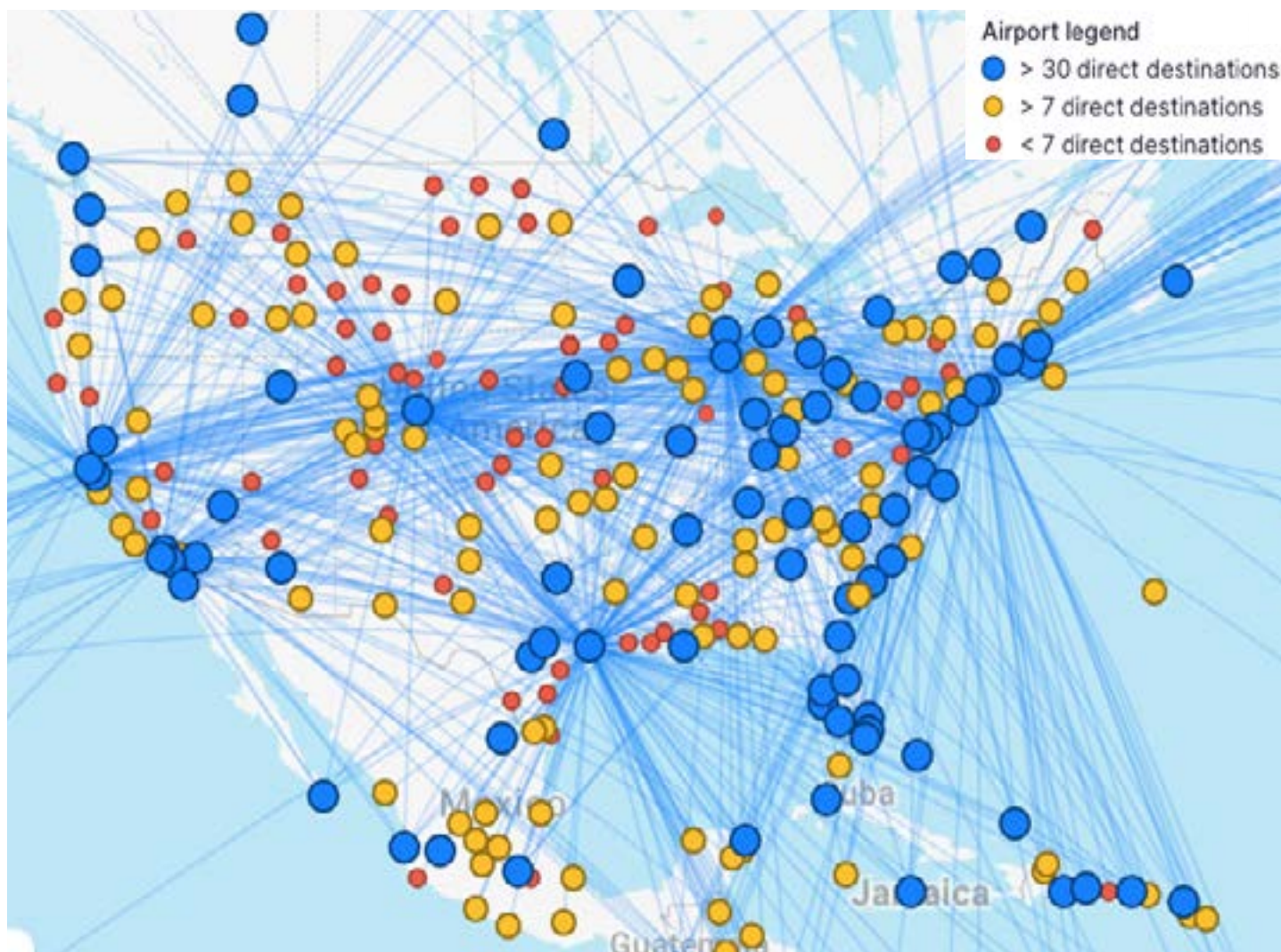
Map showing where randomly selected United 737 aircraft fly in a year, showing where data can be expected to be collected with the trace gas analyzer.
