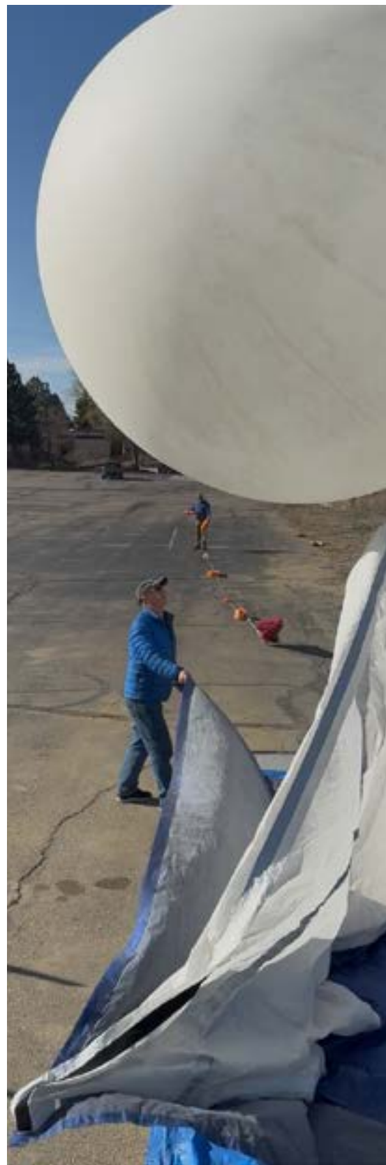
CIESRDS scientists in GML use AirCore, a balloon-borne atmospheric sampling system, to collect data on trace gases in the atmosphere from the middle stratosphere to the ground.
