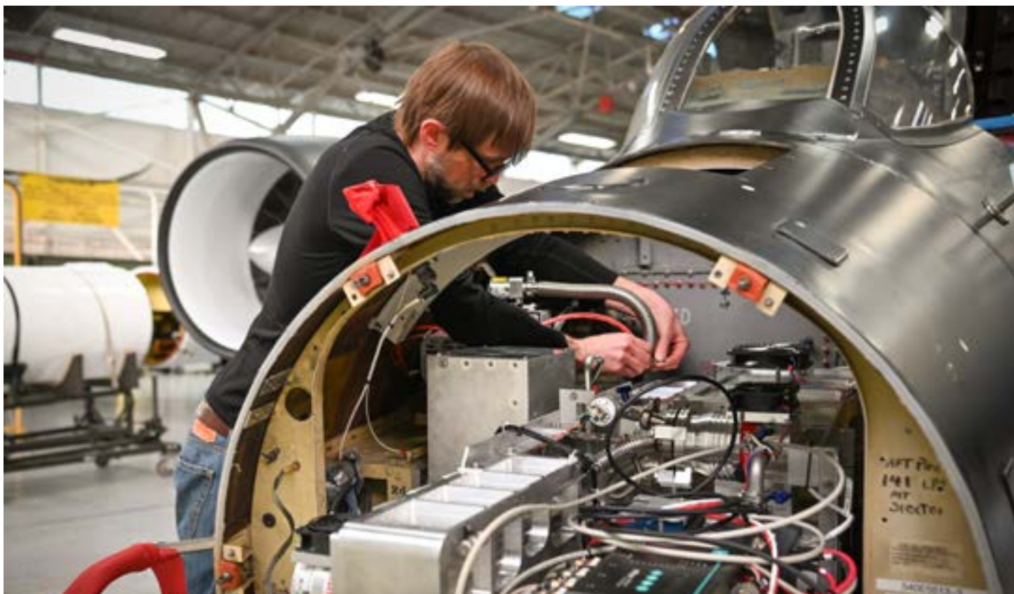
CIESRDS researcher Mike Lawler installs the PALMS (Particle Analysis by Laser Mass Spectrometry) instrument into the nose of the WB-57 for the 2022 SABRE field campaign.
