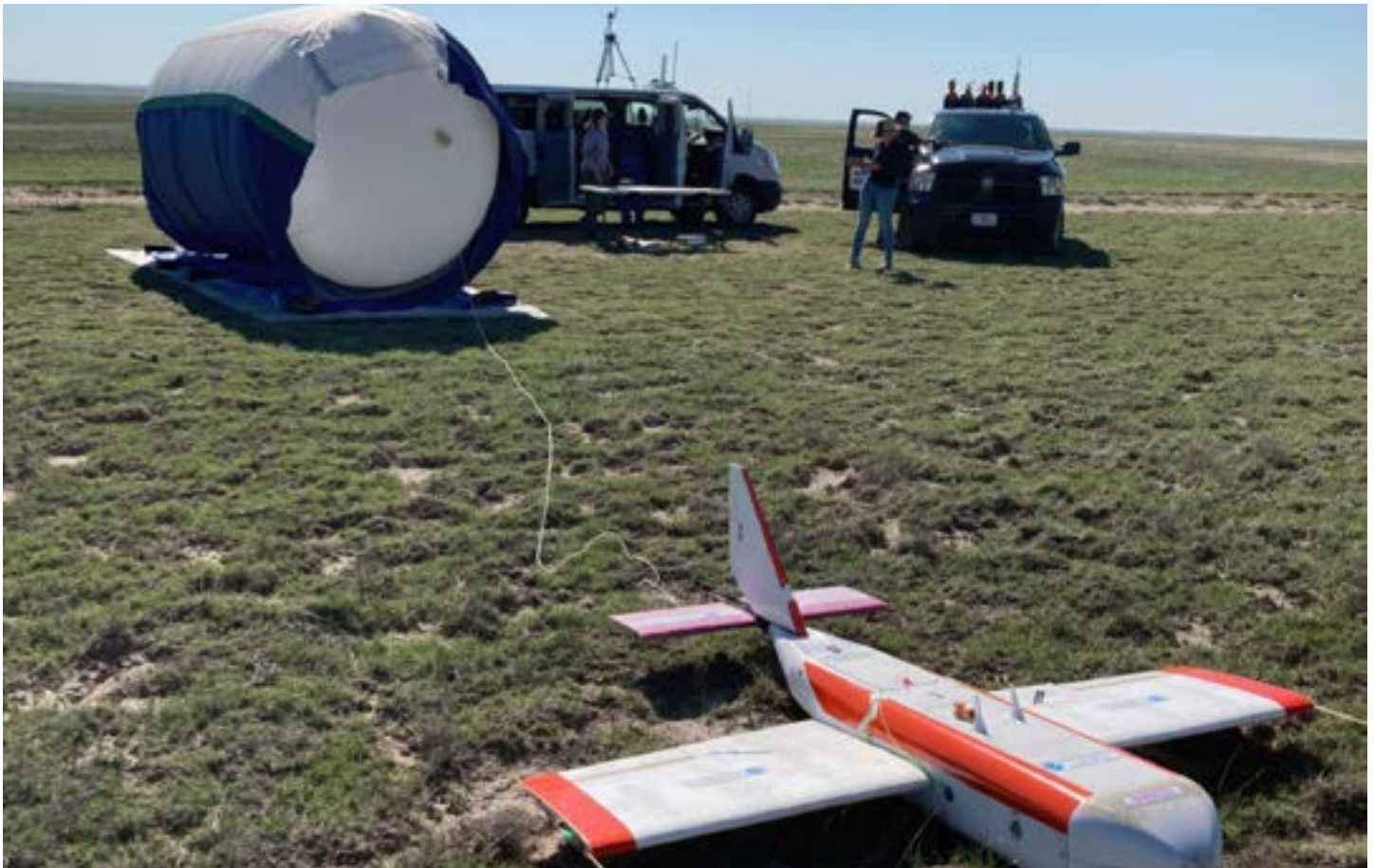
The HORUS glider and balloon prepared for a test flight on May 17, 2023 in Colorado's Pawnee National Grasslands. HORUS is a low-tech, cost-effective balloon-glider system for hosting a small payload of specialized atmospheric instruments to the edge of space, and then guiding it back to its launch location after its flight is complete.
